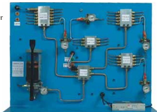
The Piping of CLHA Type Grease Lubrication System
